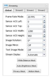
**Frame Rate Mode** - Sets the rate at which the camera's sensor will capture frames (images). For example, selecting 30 FPS means that the camera's imaging sensor will capture 30 frames per second.
