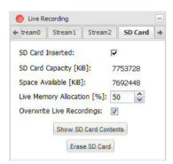
**SD Card Inserted** - Indicates the presence of an SD card in the camera. If the box is checked, an SD card is inserted. SD cards formatted with an unsupported file system will not be recognized and need to be reformatted (see "Erase SD Card" on page 54).
