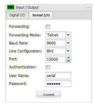
**Forwarding** - Check the **Forwarding** box to enable serial port forwarding. When forwarding is enabled, serial commands issued via TCP/IP over the designated port (see the **Port** parameter below) will be forwarded to the serial port.
