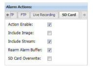
Action Enable - Check the Action Enable box on the SD Card tab to enable saving a file to the SD card as an action to take when an alarm condition is declared. The file saved to the SD card when an alarm condition is declared will be a text file that includes information such as the camera host name and the date and time.
