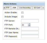
**Action Enable** - Check the **Action Enable** box on the **FTP** tab to enable the sending of an FTP upload as an action to take when an alarm condition is declared. The upload will be a text file that includes information such as the camera host name and the date and time.
