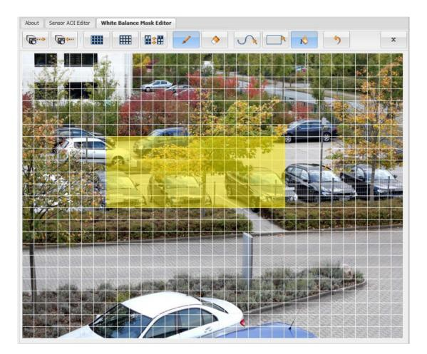
The white balance mask defines the area(s) of the image that will be used by the camera's automatic white balancing function when the **White Balance Mode** parameter is set to **Auto** (see Section 3.3 on page 13). Only the areas highlighted in the editor will be included in the white balance mask. To highlight an area within the editor, use the tools described under "Mask Editor Tools" on page 29.
