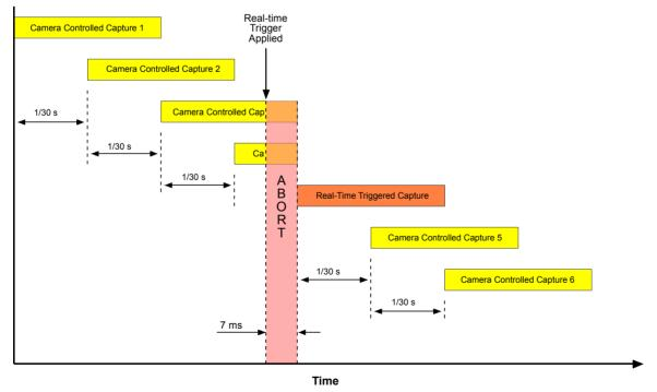
Fig. 16: Real-Time Trigger Image Capture
