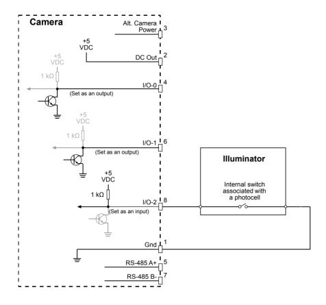
Fig. 13: Input Used to Control IR-Cut Filter Position
