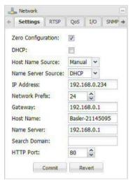
**Zero Configuration** - Check the **Zero Configuration** box to enable the camera to acquire a dynamic IP address in the 169.254.0.0/16 IP subnet, which is reserved for networking within the local network.
