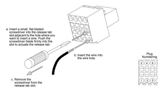
Fig. 10: Wire Insertion Method
