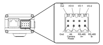
Fig. 9: Terminal Connector Pin Numbering
