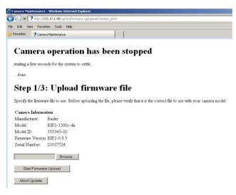
3. Use the **Browse** button in the window to select the new firmware file that you want to load onto the camera and then click the **Start Firmware Upload** button.
