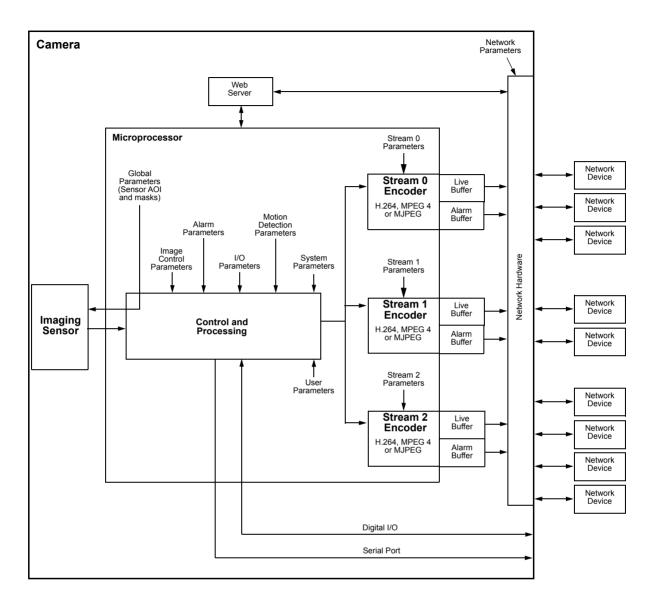
Fig. 2: Camera Block Diagram
