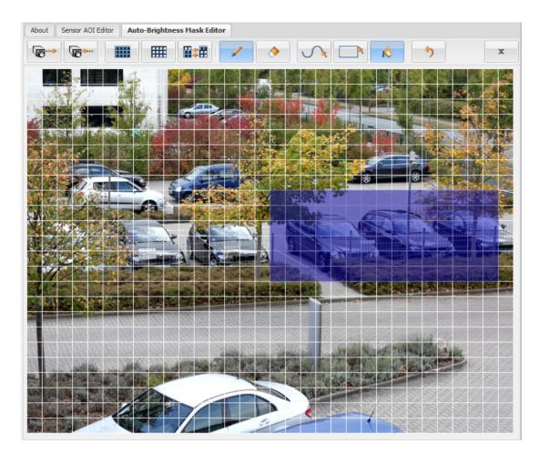
The auto brightness mask defines the area(s) of the image that will be used by the camera when it performs automatic exposure, gain, and iris control (see Section 3.3 on page 13). Only the areas highlighted in the editor will be included in the auto brightness mask. To highlight an area within the editor, use the tools described under "Mask Editor Tools" on page 29.
