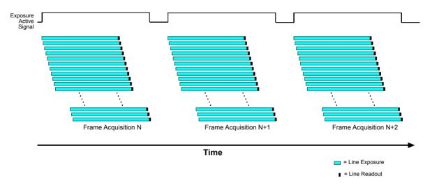
Fig. 8: Exposure Active Signal
