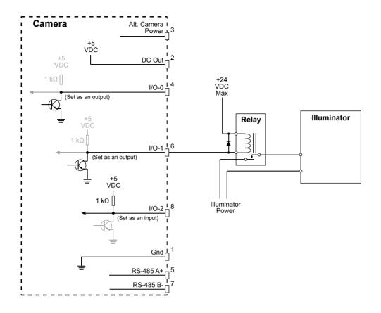
Fig. 14: Output Used to Apply Device Power
