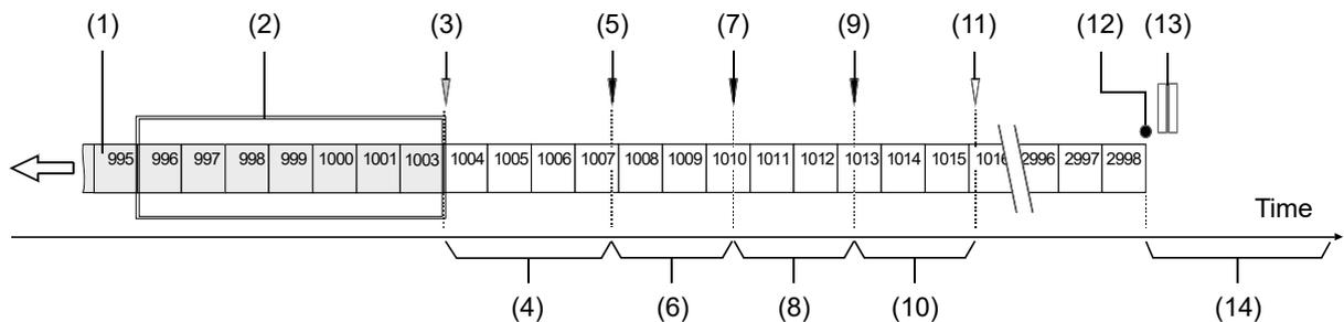
Fig. 21: Incomplete Stream of Packets and Part of the Resend Mechanism
