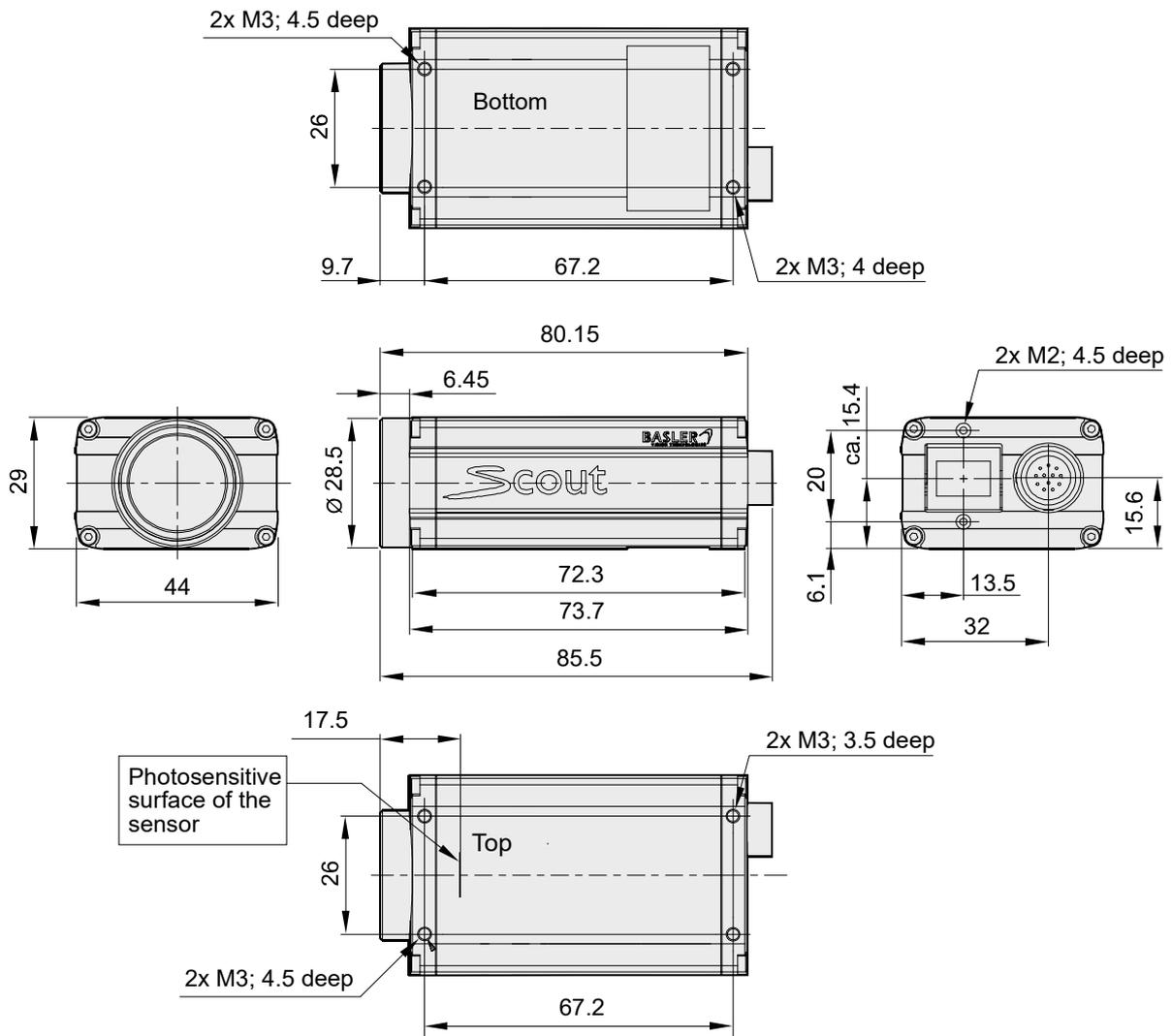
Fig. 13: Mechanical Dimensions (in mm) for Cameras with the Standard C-mount Lens Adapter
