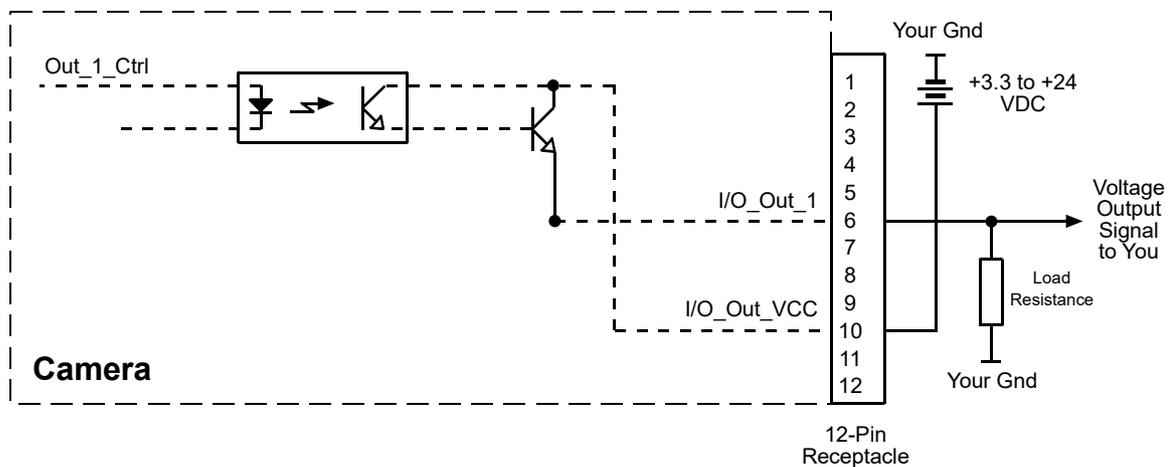
Fig. 31: Typical Voltage Output Circuit
