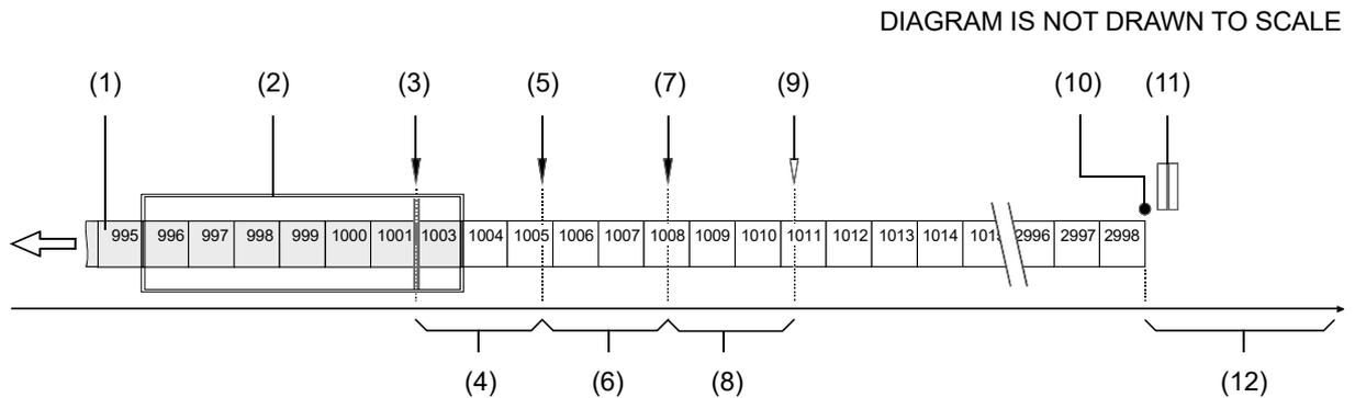
Fig. 22: Combination of Threshold Resend Mechanism and Timeout Resend Mechanism
