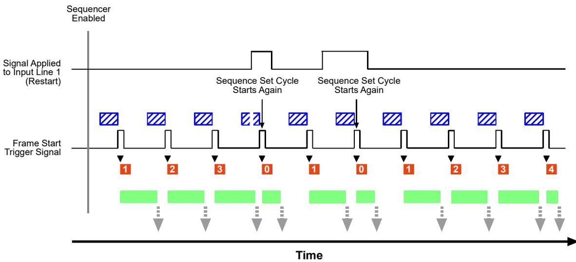
Fig. 67: Sequencer in Controlled Sequence Advance Mode with Always Active as the Sequence Control Source and Synchronous Restart Controlled by Line 1
