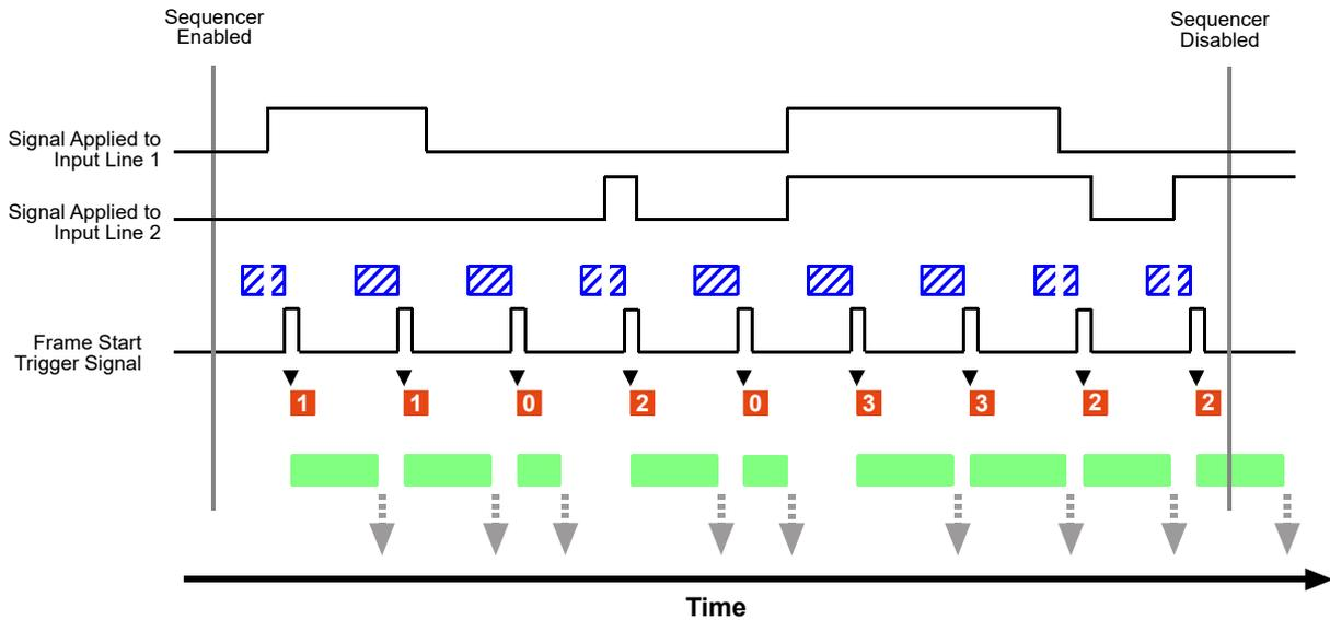
Fig. 71: Sequencer in Free Selection Mode
