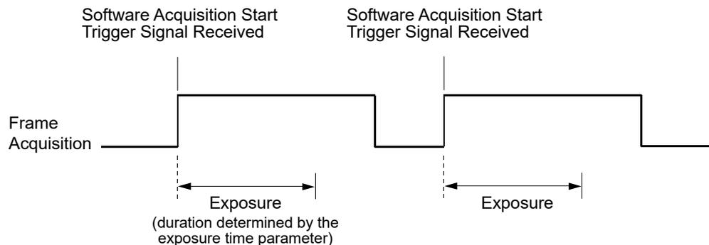
Fig. 42: Frame Acquisition with a Software Acquisition Start Trigger
