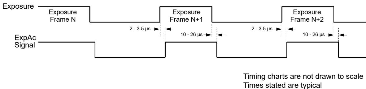
Fig. 54: Exposure Active Signal
