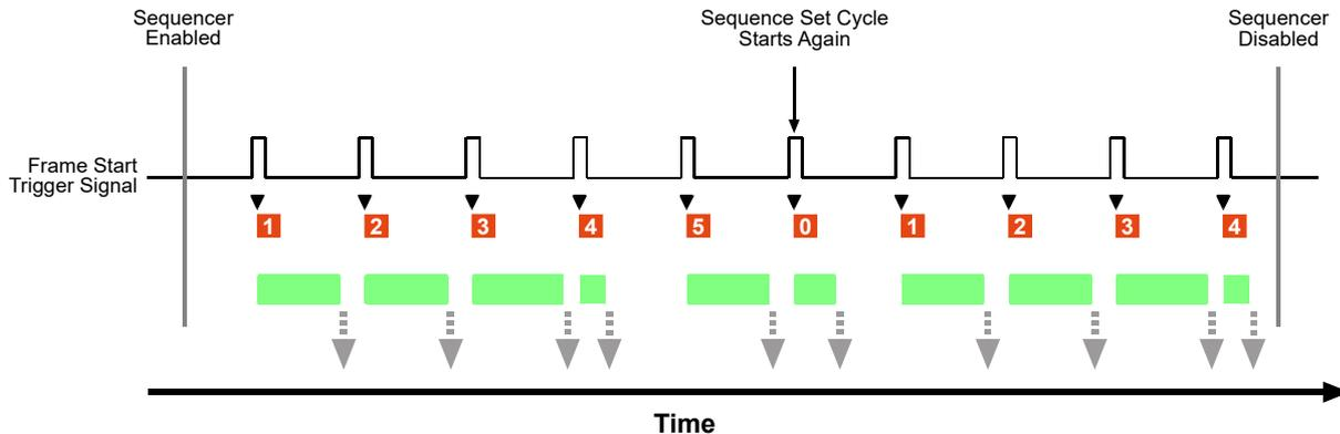
Fig. 66: Sequencer in Controlled Sequence Advance Mode with Always Active as the Sequence Control Source
