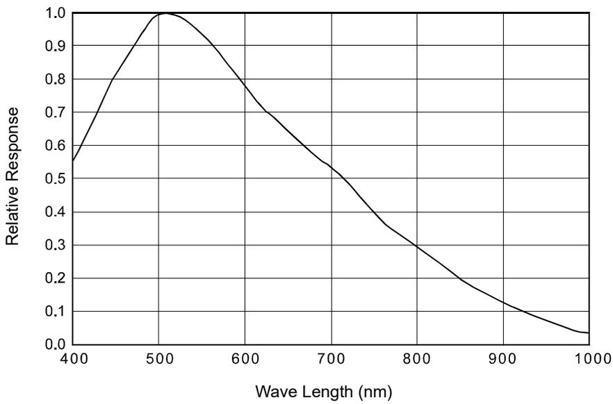
Fig. 3: scA1000-30gm Spectral Response
