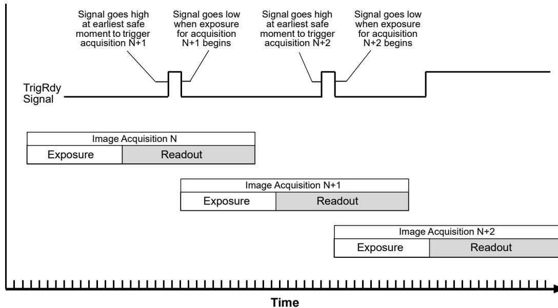
Fig. 55: Trigger Ready Signal
