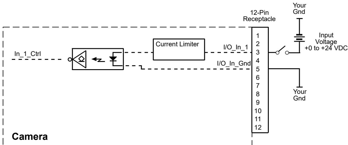
Fig. 30: Typical Voltage Input Circuit
