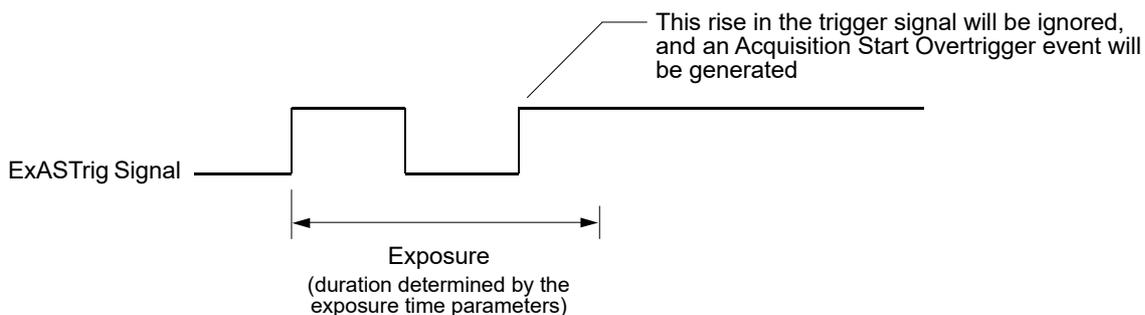
Fig. 44: Overtriggering with Timed Exposure
