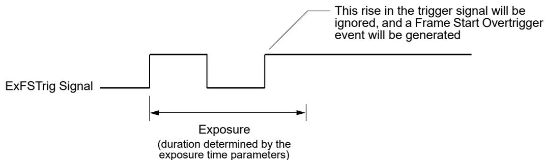
Fig. 40: Overtriggering with Timed Exposure
