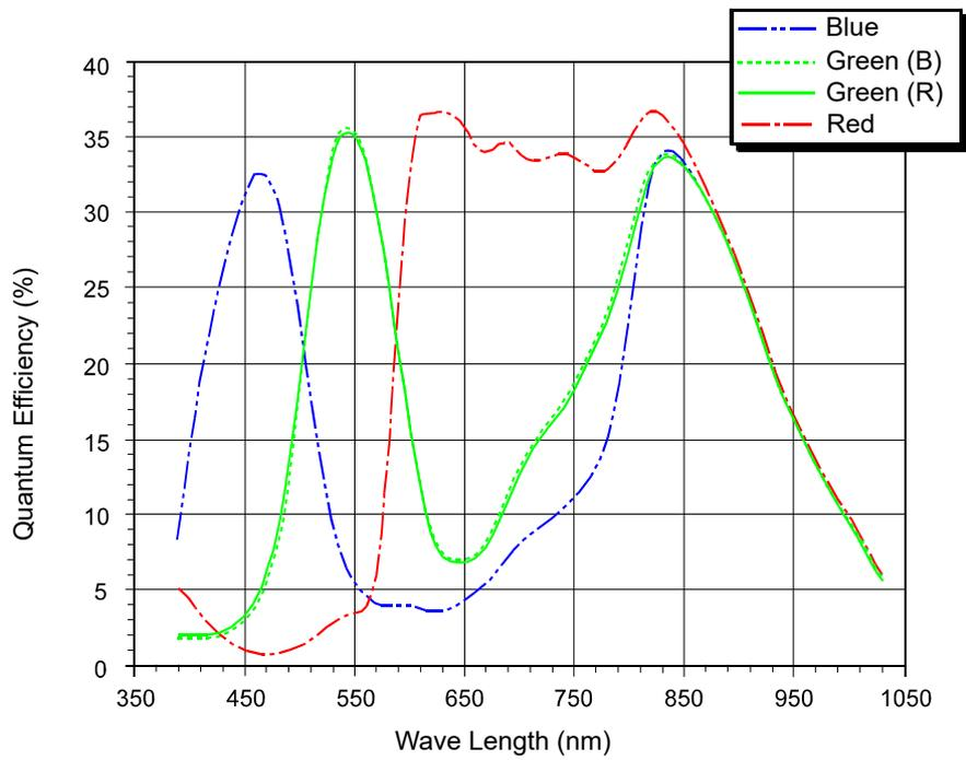
Fig. 8: scA750-60gc Spectral Response
