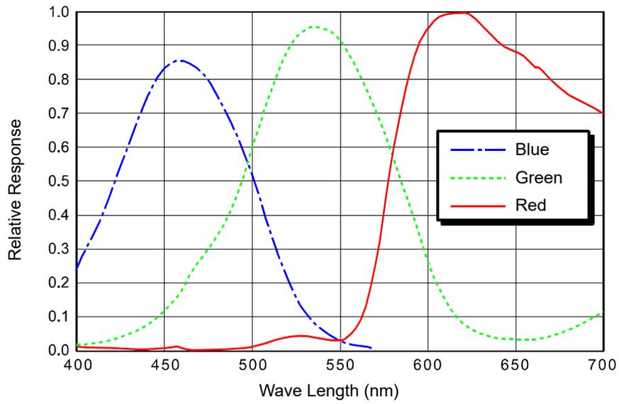
Fig. 12: scA1600-14gc and scA1600-28gc Spectral Response
