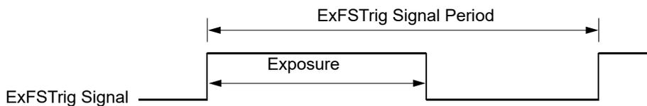
Fig. 41: Trigger Width Exposure with Rising Edge Triggering
