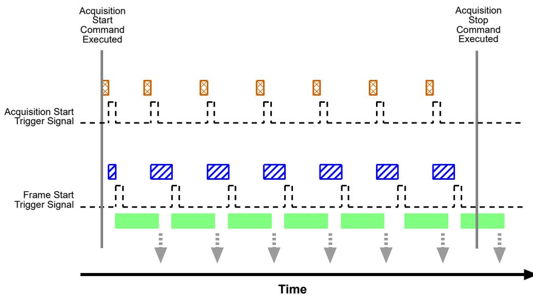
Fig. 47: Use Case 1 - Acquisition Start Trigger Off and Frame Start Trigger Off
