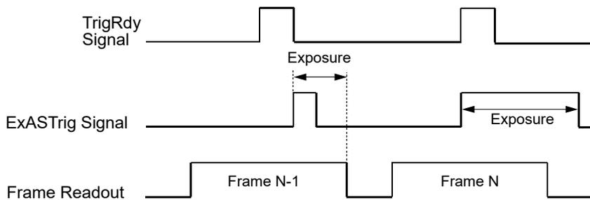
Fig. 46: Trigger Width Exposure Mode with Overlapped Exposure
