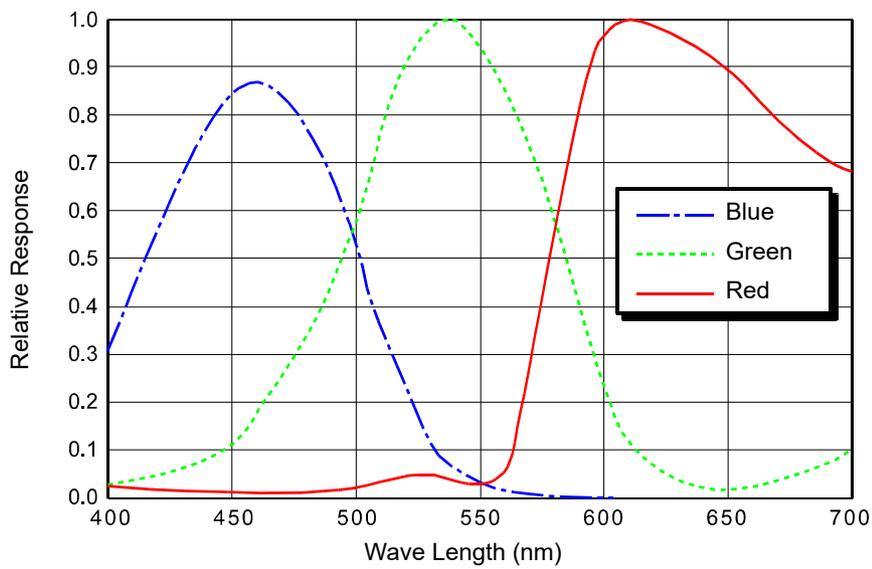
Fig. 9: scA1000-30gc Spectral Response
