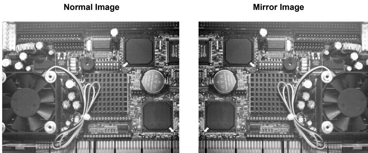
Fig. 74: Reverse X Mirror Imaging
