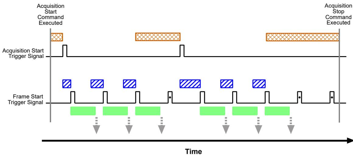
Fig. 37: Acquisition Start and Frame Start Triggering
