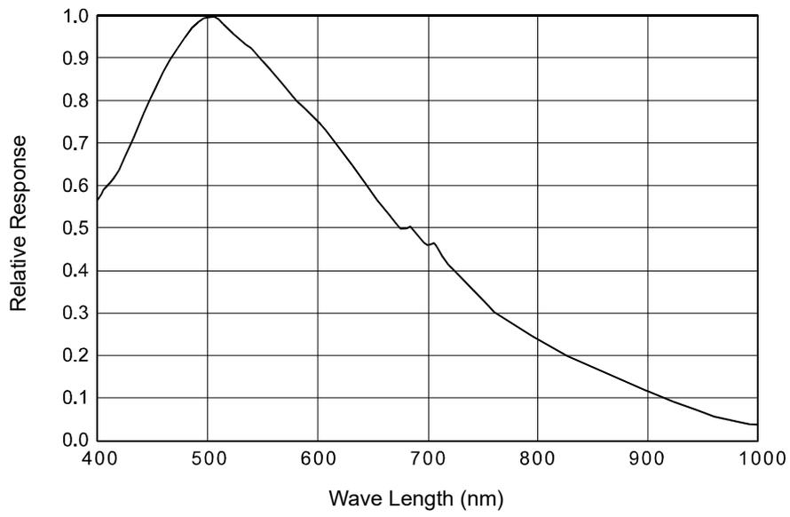
Fig. 6: scA1600-14gm and scA1600-28 gm Spectral Response
