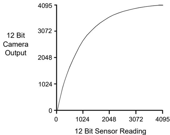
Fig. 77: Lookup Table with Values Mapped for Higher Camera Output at Low Sensor Readings
