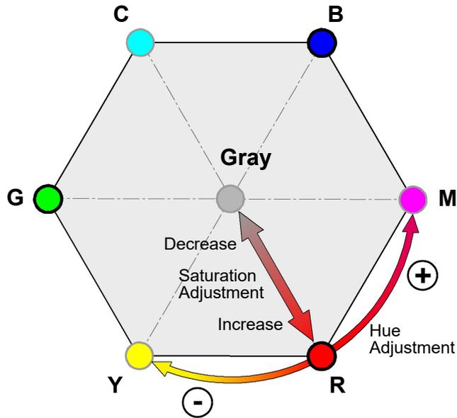
Fig. 61: Hue and Saturation Adjustment In the Color Hexagon. Adjustments Are Indicated for Red as an Example
