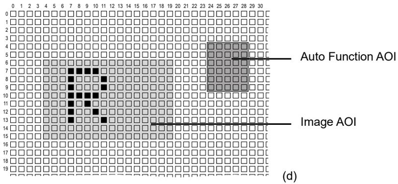
Fig. 81: Various Degrees of Overlap Between the Auto Function AOI and the Image AOI
