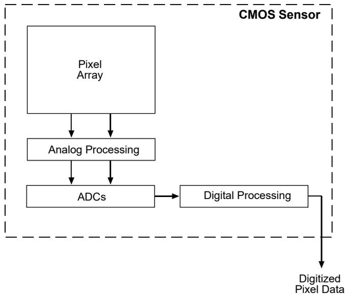
Fig. 26: CMOS Sensor Architecture
