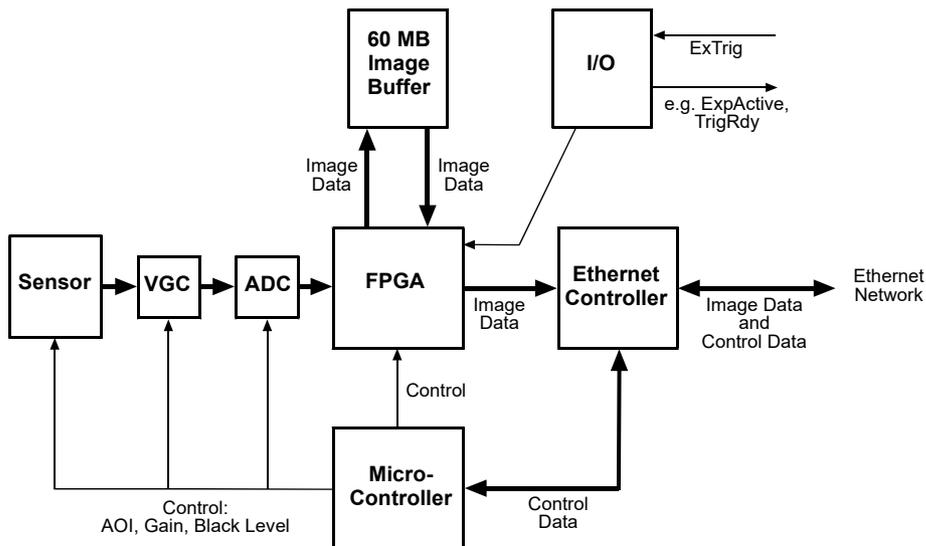
Fig. 25: Camera Block Diagram
