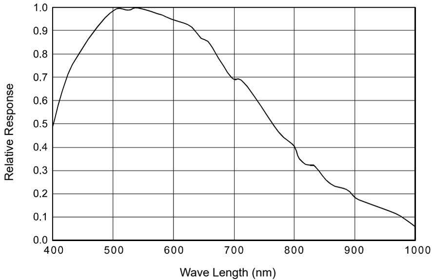
Fig. 5: scA1400-17gm and scA1400-30gm Spectral Response
