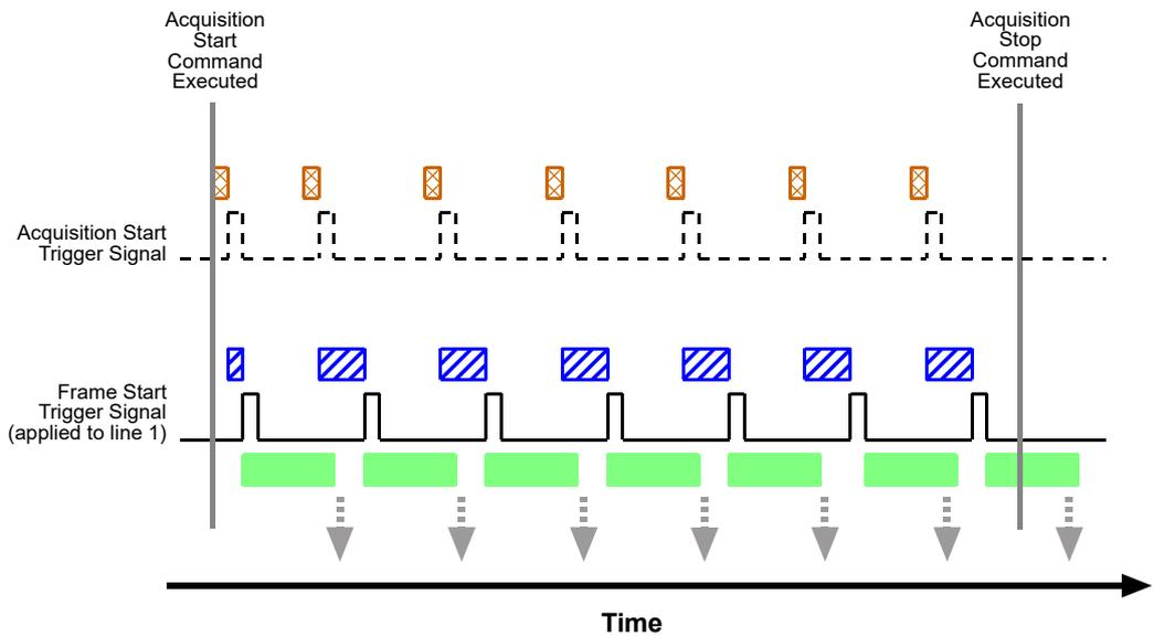
Fig. 48: Use Case 2 - Acquisition Start Trigger Off and Frame Start Trigger On
