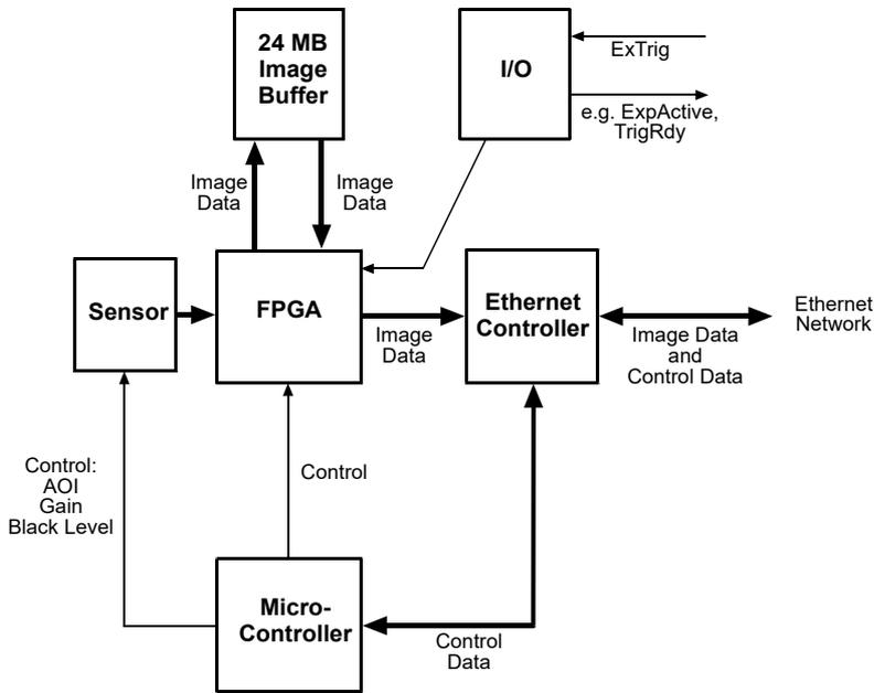
Fig. 27: Camera Block Diagram
