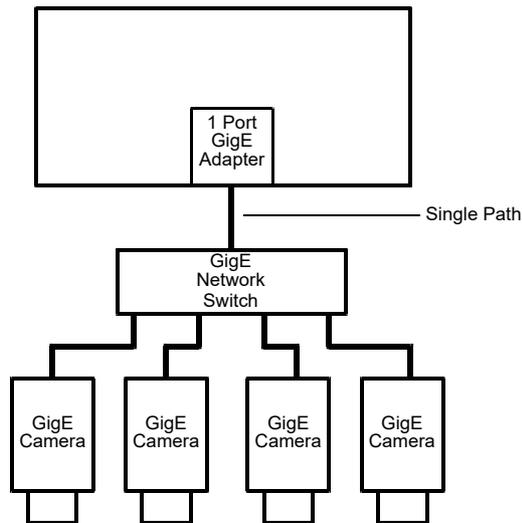
Fig. 23: Multiple Cameras on a Network
