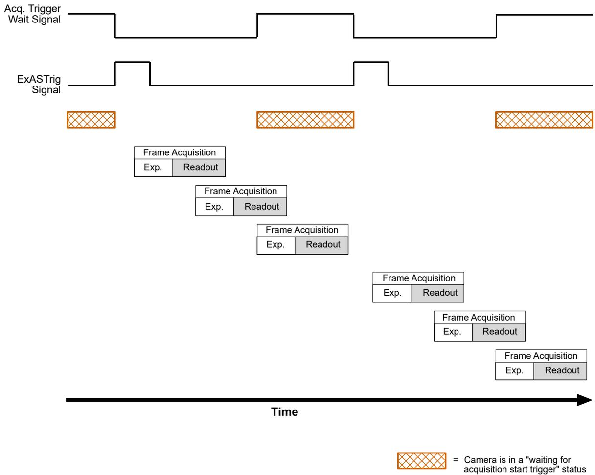
Fig. 57: Acquisition Trigger Wait Signal
