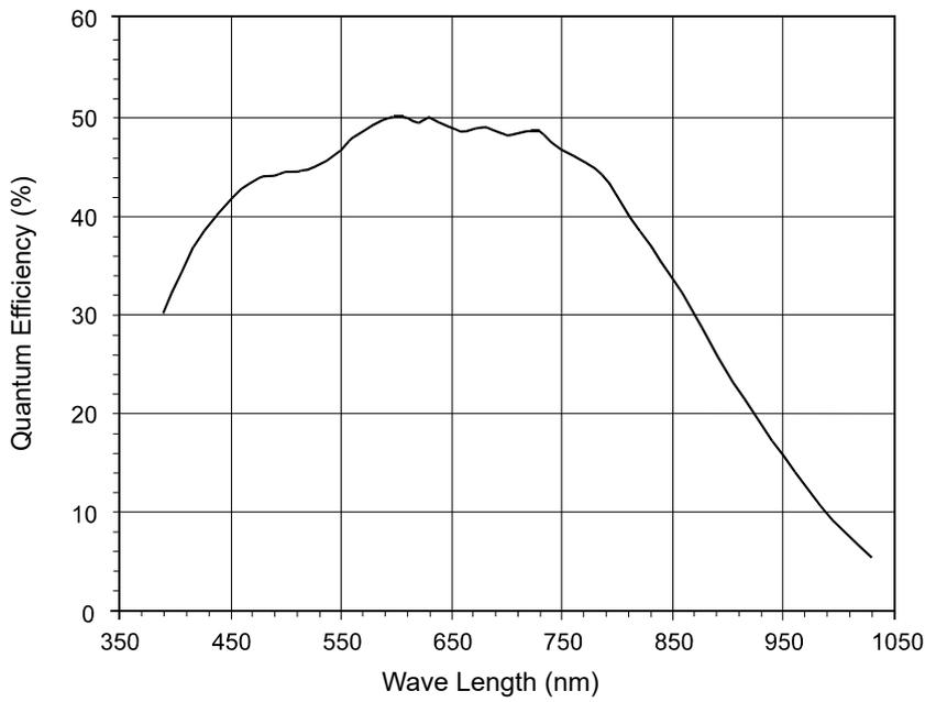
Fig. 2: scA750-60gm Spectral Response
