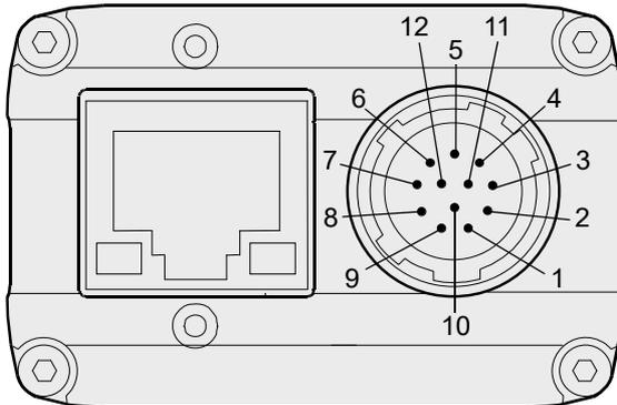
Fig. 29: Pin Numbering for the 12-pin Receptacle
