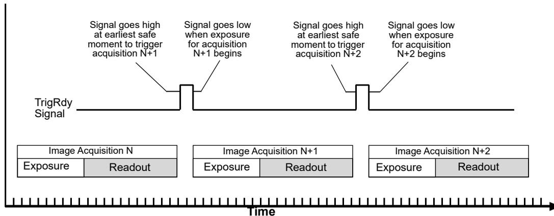
Fig. 56: Trigger Ready Signal
