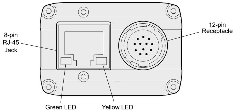
Fig. 28: Camera Connectors and LED
