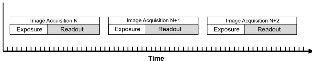
Fig. 51: Non-overlapped Exposure
