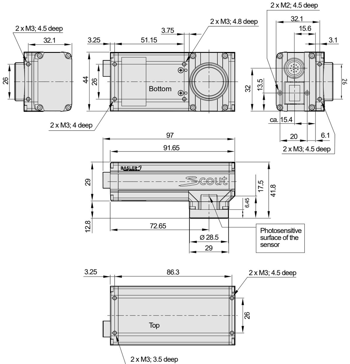
Fig. 17: Mechanical Dimensions (in mm) for Cameras (90° Head) with the Standard C-mount Lens Adapter
