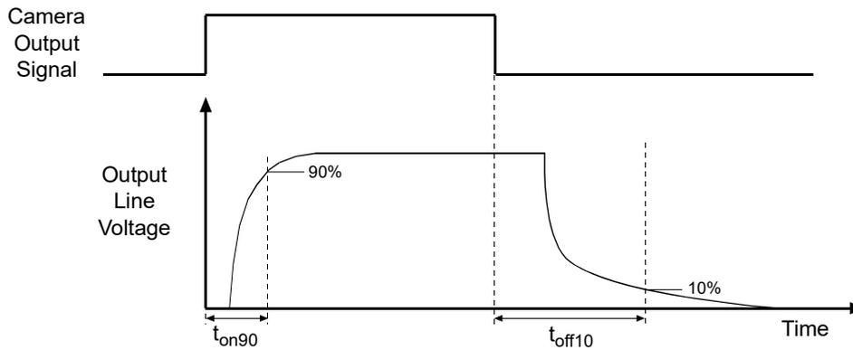
Fig. 32: Output Line Response Times
