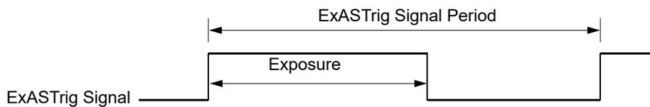
Fig. 45: Trigger Width Exposure with Rising Edge Triggering
