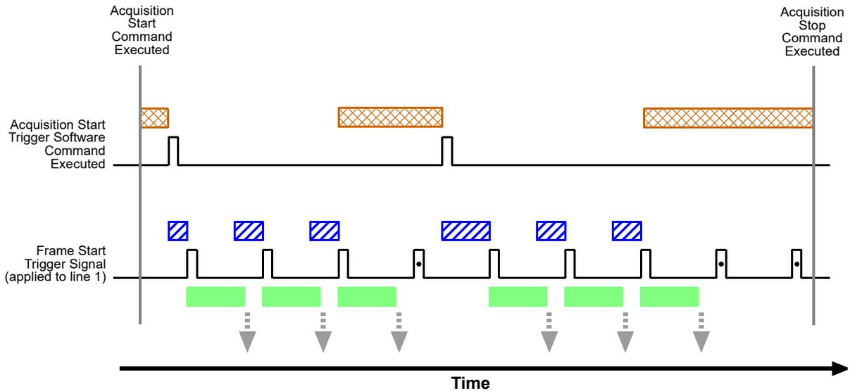
Fig. 50: Use Case 4 - Acquisition Start Trigger On and Frame Start Trigger On
