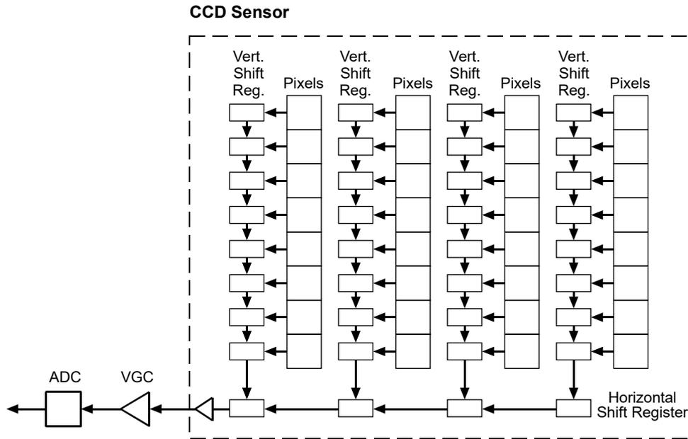
Fig. 24: CCD Sensor Architecture
