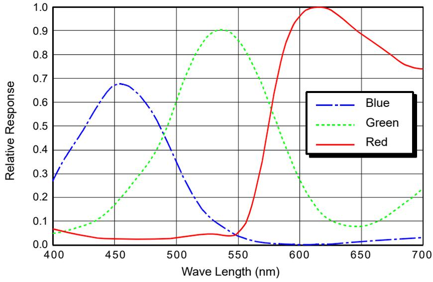
Fig. 10: scA1300-32gc Spectral Response
