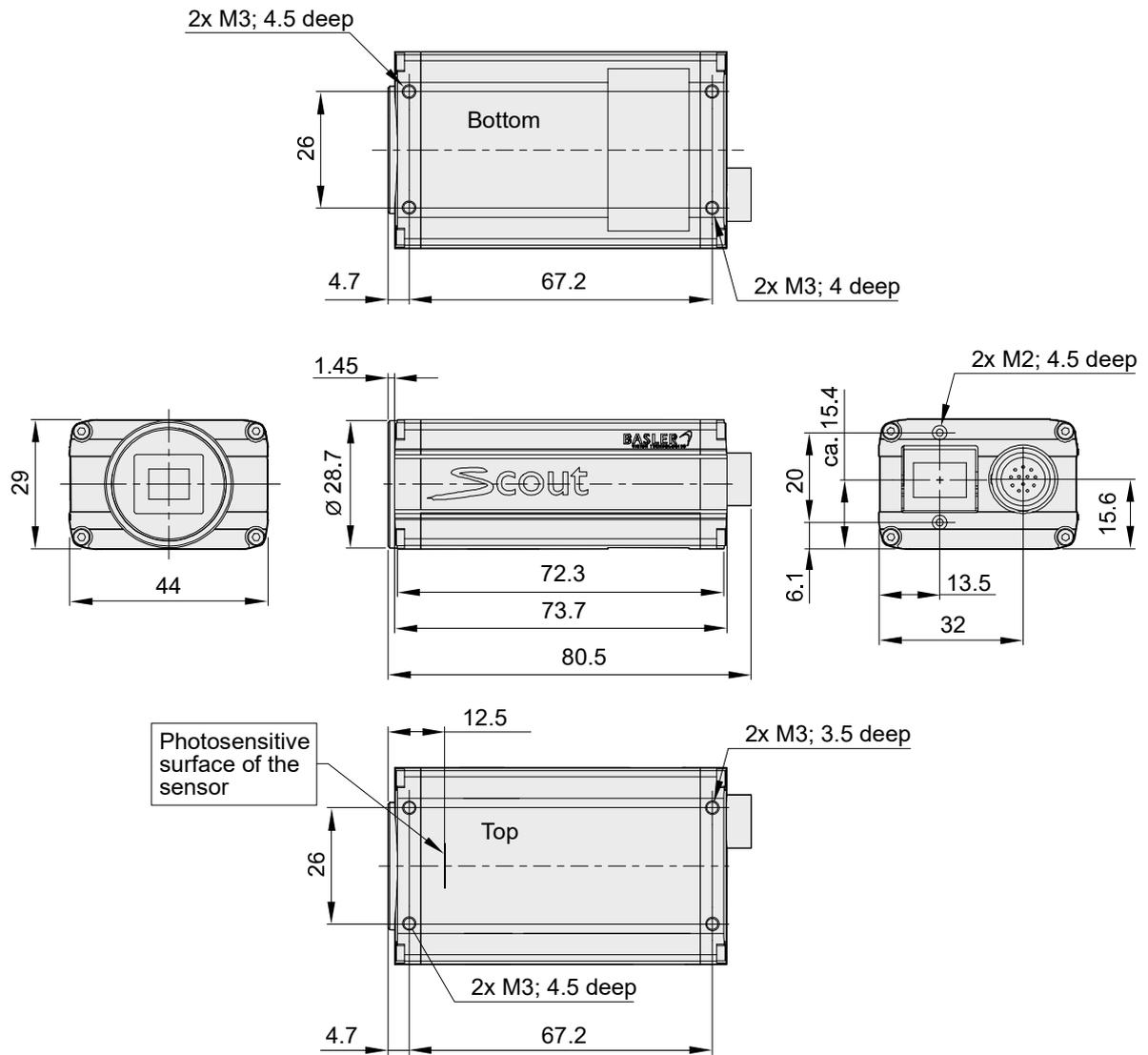
Fig. 14: Mechanical Dimensions (in mm) for Cameras with an Optional CS-mount Lens Adapter
