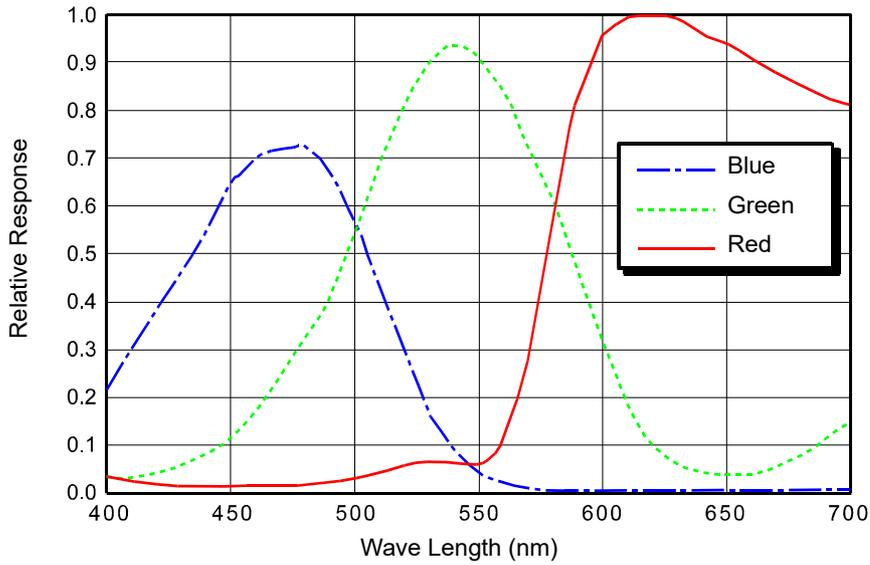
Fig. 11: scA1400-17gc and scA1400-30gc Spectral Response
