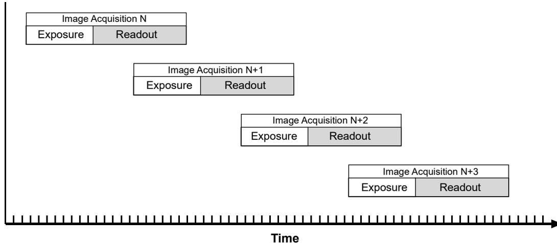
Fig. 52: Overlapped Exposure
