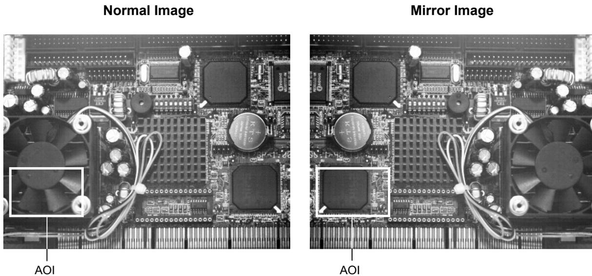
Fig. 75: Using an AOI with Reverse X Mirror Imaging
