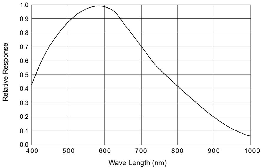
Fig. 4: scA1300-32 gm Spectral Response
