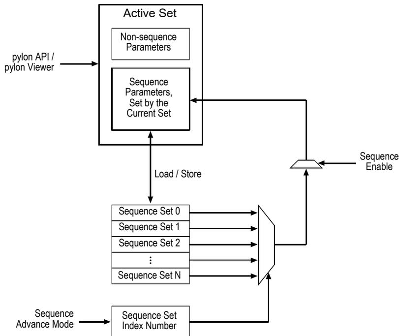
Fig. 64: Sequence Feature Block Diagram
