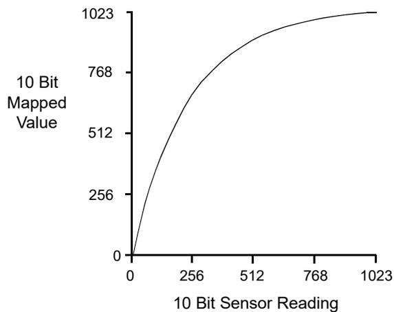
Fig. 79: Lookup Table with Values Mapped for Higher Camera Output at Low Sensor Readings
