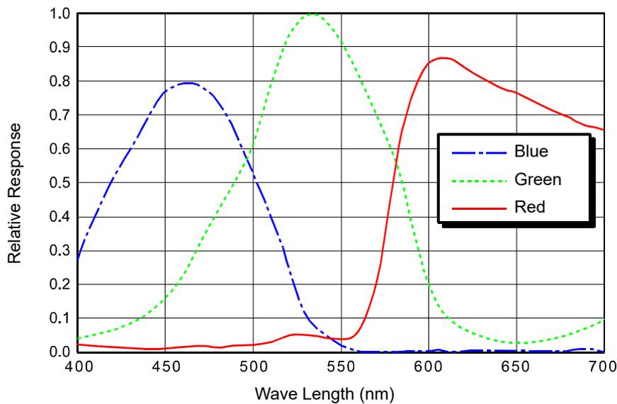
Fig. 7: scA640-70gc Spectral Response
