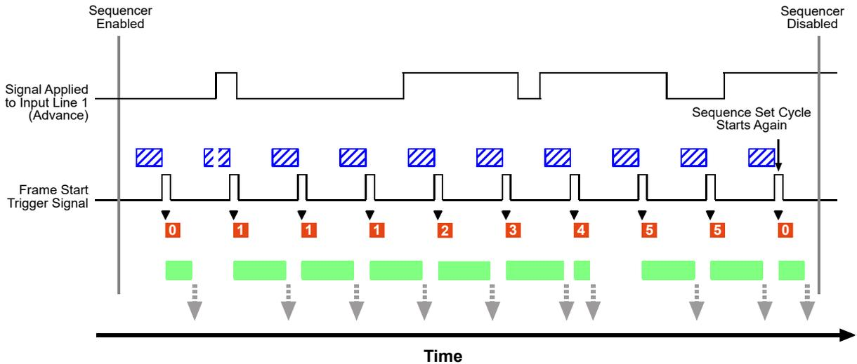
Fig. 68: Sequencer in Controlled Sequence Advance Mode with Line 1 as the Sequence Control Source
