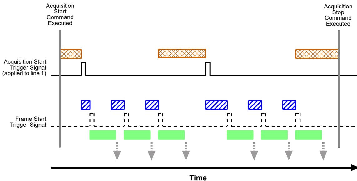
Fig. 49: Use Case 3 - Acquisition Start Trigger On and Frame Start Trigger Off
