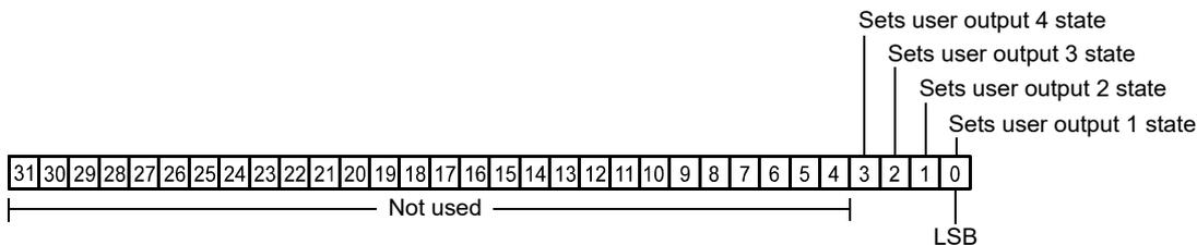
Fig. 34: User Output Value All Parameter Bits
