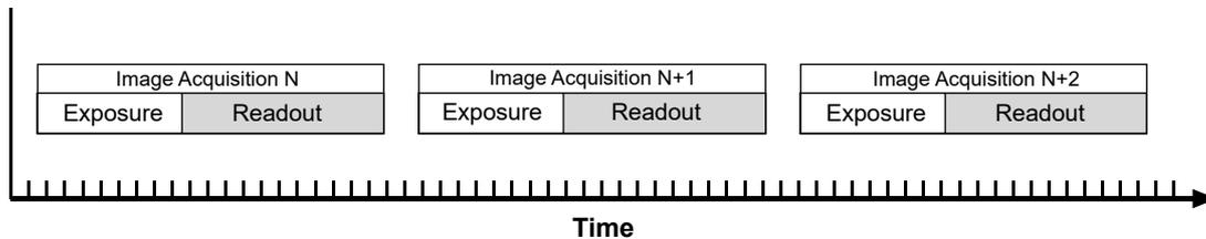
Fig. 53: Non-overlapped Readout and Exposure
