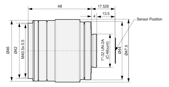
Not to scale Dimensions in mm  $\rightarrow$  Download the CAD/technical drawing for your Basler Lens [].
