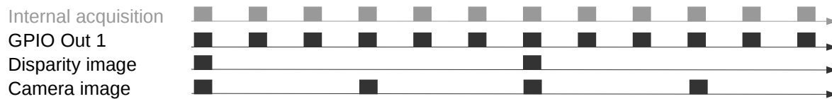
Fig. 6.35: Example of using the ExposureActive mode for GPIO Out 1 with a user-defined frame rate of 8 Hz. The internal image acquisition is always 25 Hz. GPIO Out 1 is HIGH for the exposure time of every image. A disparity image is computed for camera images that are sent out via GigE Vision according to the user-defined frame rate.
