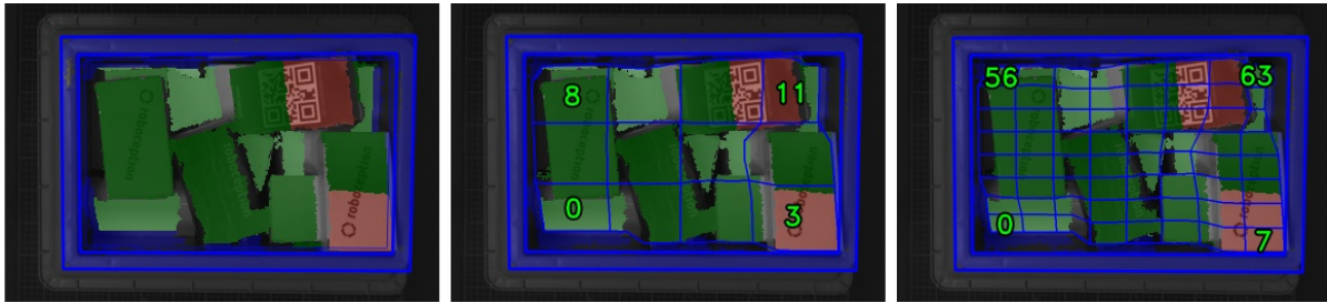
Fig. 6.10: Visualizations of the load carrier filling level: overall filling level without grid (left), 4x3 grid (center), 8x8 grid (right). The load carrier content is shown in a green gradient from white (on the load carrier floor) to dark green. The overfilled regions are visualized in red. Numbers indicate cell IDs.
